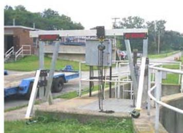
GANTRY showing height difference with legs and reducing span with Beam over hanging left leg
