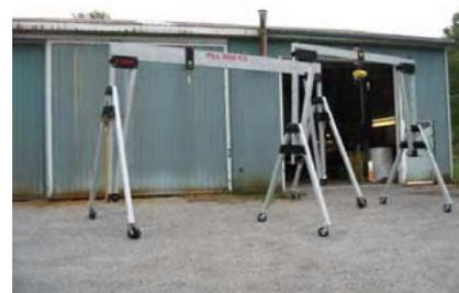
eme 6600R at min lift height, 1100R at max lift height
